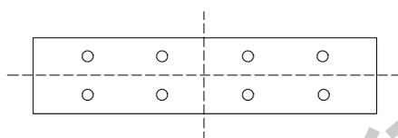
图3 条缝形风口测点布置
